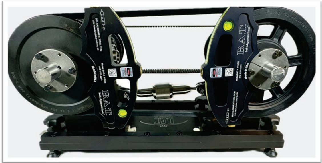
i. Picture of B.A.T “V”-Belt Alignment:
